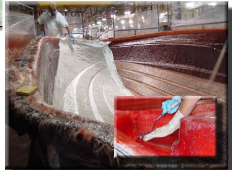
Hand lay up to make the preformed racket
