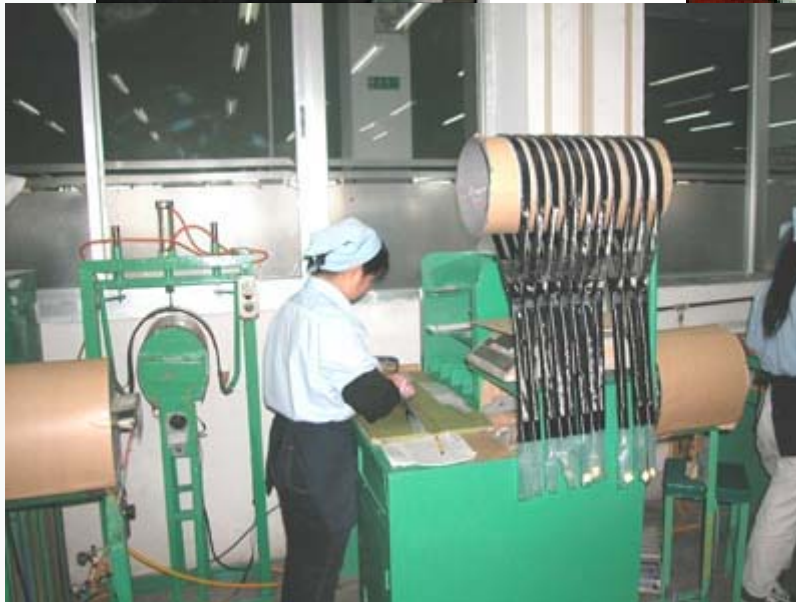
Hand lay up to make the preformed racket
