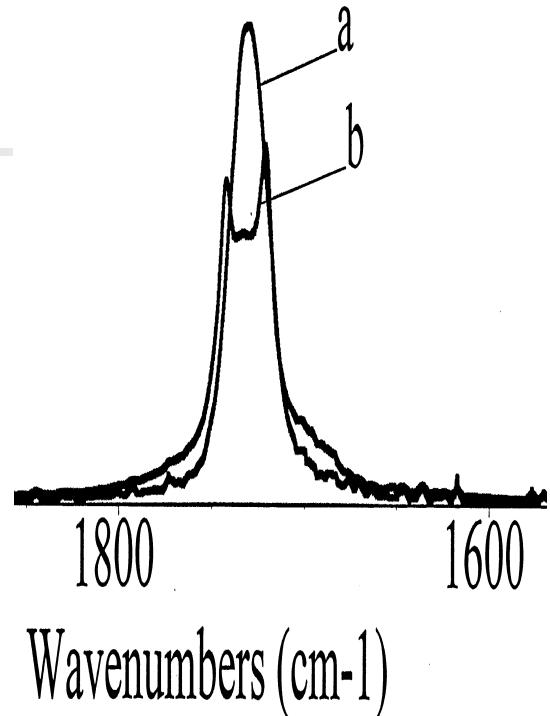
Comparison between the theoretical spectrum of the blend and the real spectrum in the zone of the carbonyl group: a) PCL/PVC, 25%; b) simulation of PCL/PVC, 25%.
