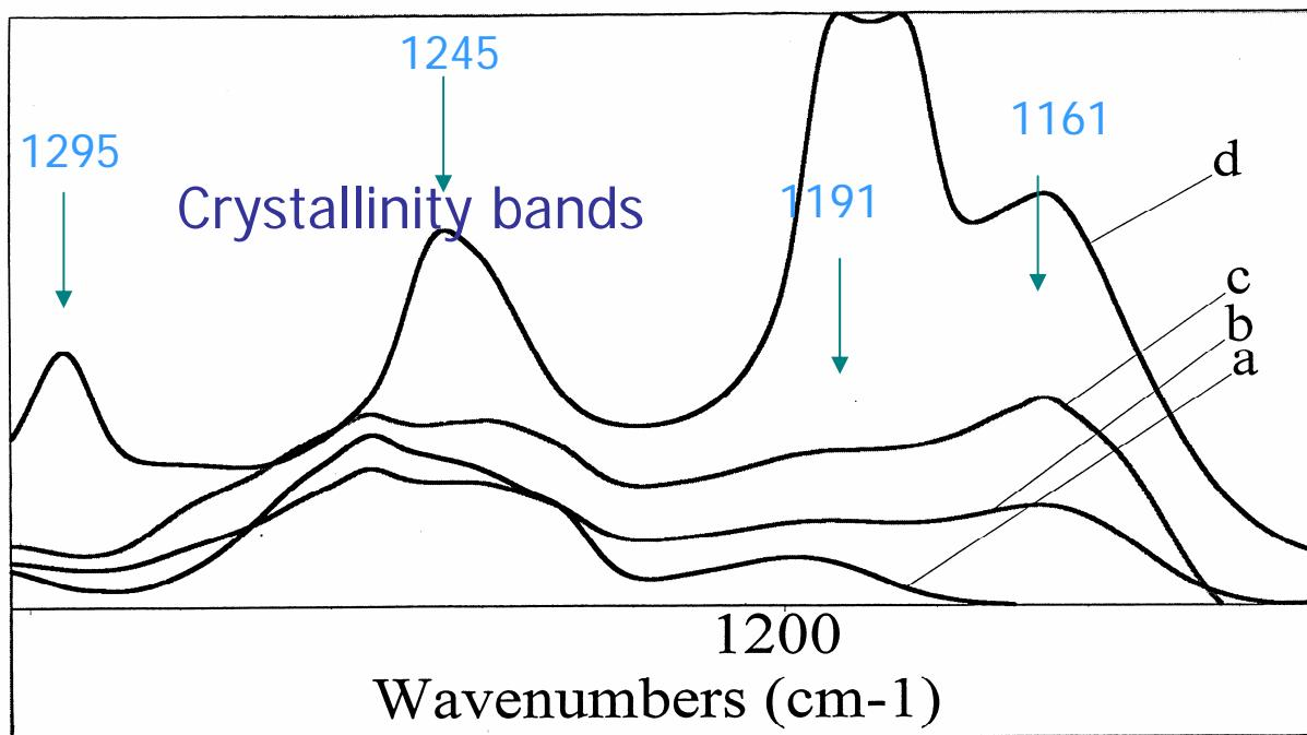
Spectra of blends in the zone of 1100-1300 cm<sup>-1</sup>; a) PVC film; b) PCL/PVC, 10%; c) PCL/PVC, 50 %; d) PCL film.
