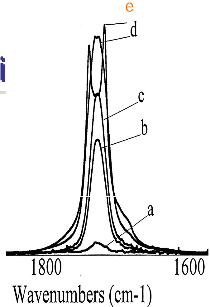
Spectra of blends in the zone of the carbonyl group: a) PVC film; b) PCL/PVC, 10%; c) PCL/PVC, 25%; d) PCL/PVC, 50%; e) PCL film
