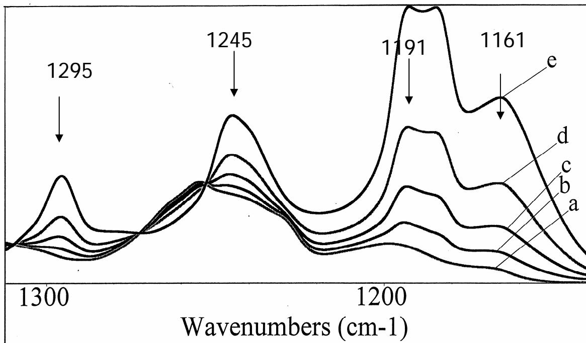
Simulated spectra of blends in the zone 1100-1300  $\text{cm}^{-1}$ : a) PVC film; b) simulation PCL/PVC, 10%; c) simulation PCL/PVC, 25%; d) simulation PCL/PVC, 50%; e) PCL film.
