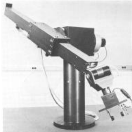
Fig. 1.11 The Stanford Arm. Photo courtesy of the Coordinated Science Lab, University of Illinois at Urbana-Champaign.
